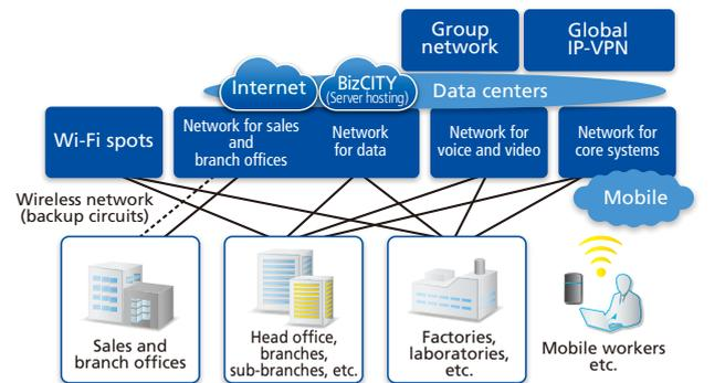
Enhanced network reliability through segmentation according to usage (core, data or voice/video)
