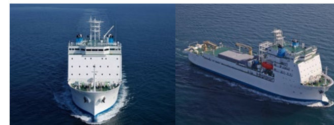
Cable-Laying Ship Kizuna Total tonnage: 8,598 tons; deadweight capacity: 4,098 tons, total length: 108.64 meters; width: 20 meters; designed load draft: 6.0 meters; sea speed: 13.2 knots; maximum passenger capacity: 60; cruising distance: 9,500 nautical miles (around 30 days); registry location: Japan (Tokyo)
