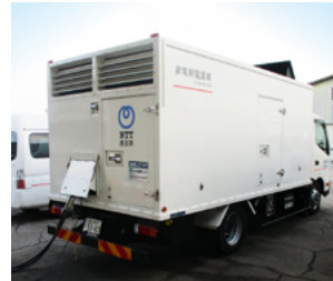
[ NTT West's emergency power supply vehicle ]
