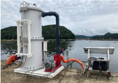
[ Oxygen fighter® (left) and box containing ICT buoy communication equipment (right) ]
