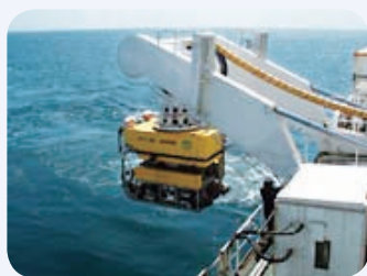
ROV capable of submerging to a depth of 2,500 meters
