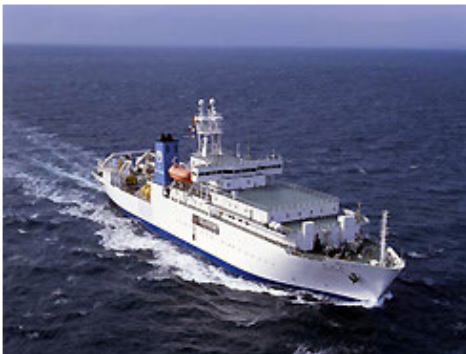
■ The Subaru, a vessel that lays submarine cable (total weight: 9,557 tons)
