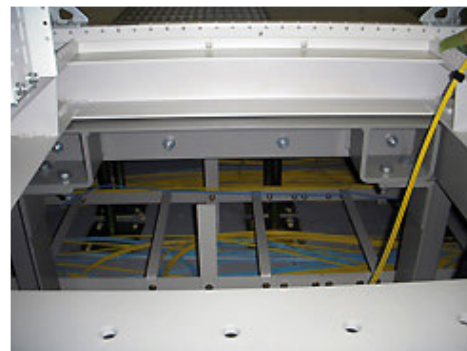
■ Wiring layout with dual-walled structure (underfloor)
