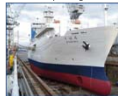
After hull painting
