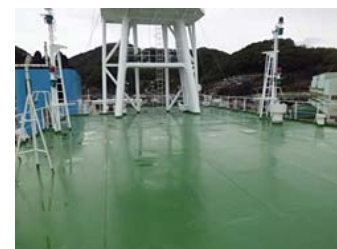
After heat-shield painting
