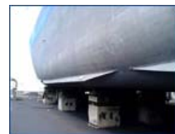
After hull sandblast painting
