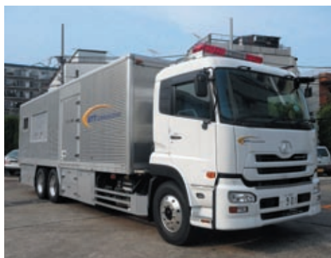
■ Mobile power supply truck
